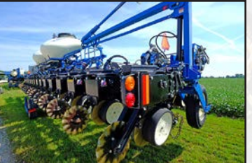
2011 KINZE 3600 ASD 32 row bean planter w/brush meters, no till coulters, Martin spaders w/drag chains, Keeton seed firmers
