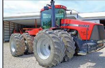
2003 CASE IH STX425 w/3672 hours, radar, scraper hitch, diff locks, 20 front weights, 710/70/R42 tires, SN SNJEE0102500
