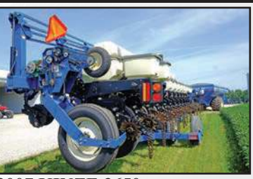
2007 KINZE 3650 16 row corn planter, liq. fert. w/ground driven pump, HD single disc fert. openers, finger pickup row cleaners, new seed openers, pop-up fert., two 8 row CD's, squeeze pumps, Martin row cleaners, Martin spader closing wheels w/drag chains, KPM 2 monitor, Keeton seed firmers
