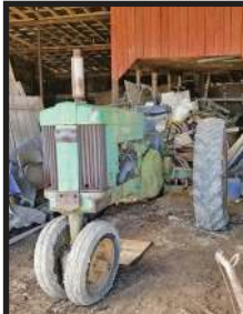
JOHN DEERE 60 TRACTOR Narrow front end, gas, 3 pt, 540 pto, 1 hyd. remote, 13.6-38 rear tires
