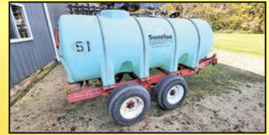
1000 gallon nurse trailer , 2" plumbing with pump
