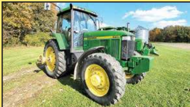
1998 JD 7810 Tractor , MFWD, 4053 hours, one owner, 16 speed PQ trans., 540/1000 PTO 18.4-42 axle duals, 14.9-30, fenders 3 SCV, radar, quick hitch, 12 frt. Wts. SN: RW7810H014980
