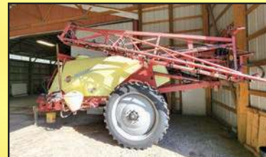
Hardi Navigator 3000 , 800 gallon sprayer, 60 ft. boom, 3 way nozzle body, 12.4-42 tires, 540 PTO pump "rebuilt", SN: 311100859
