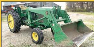
1968 JD 4000 Diesel Tractor , w/ JD 720 loader, syncro range trans, 1 SCV, 15.5-38 rear tires, 9.5L-15, 72" bucket, hours unknown, tach not working, SN: B213R 221557R
