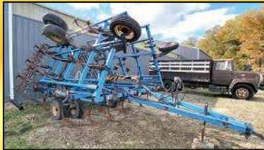
DMI Tiger Mate II , 24 ft. Field cultivator, Nicol knock-on sweeps, tandems on wings, with 5-bar spike harrow and rear hitch, SN: 822146
