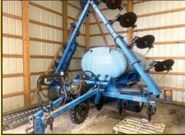
DMI 2800 13 knife liquid fertilizer tool bar, John Blue pump, 800 gallon tank, 14L-16.1, SN: JFH0010955
