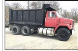
**1987 GMC BRIGADIER DUMP TRUCK**, 726,396 miles, tandem axle, air brakes, coal chute, 11r-22.5 tires, #1GDS9C4C8HV526746
