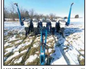
**KINZE 3000** 6/11 row no till planter, 15"/30" spacing, poly box extensions, keeton seed firmers, 1 Martin spike 1 rubber closing wheel on each row, 6 extra boxes with corn meters nice well kept planter, #642623
