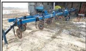
**DALTON AG PRODUCTS D3035**, 15 knife 3pt. liquid applicator, Raven flow meter with half width shut-off, monitor not included, no-till coulters, hyd. fold wings and end transport for storage, #10251
