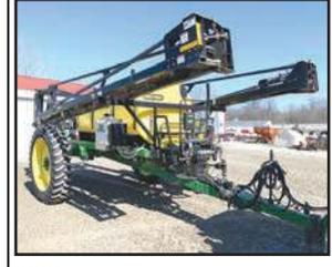
**2006 BESTWAY FIELD PRO IV 1200**, 1200 gallon pull type sprayer. 80ft. boom, 20 spacing, triple nozzle body, newer Tee Jet 11004 tips, fence row nozzle, 5 section shut off, auto boom height, JD rate controller (no display), chemical inductor, rinse tank, foam marker, 14.9R46 tires, #212223
