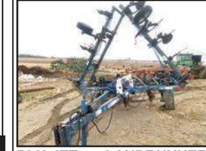
**BLU-JET LANDRUNNER**, 15 knife pull type anhydrous applicator, coulter with mole knife, Raven accuflow super cooler with SCS440 control box
