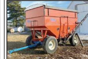
**KILLBROS 390** wagon, 2 compartment, 15' poly hyd. Seed auger, telescoping seed tube, augermate w/Honda electric start engine, roll tarp, #D47530109
