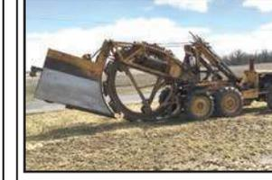
**SPEICHER 600 TRENCHER**, 1,489 hrs, 6 cylinder gas engine, grade stakes, 12.4-24 tires, good cables, chains, and sprockets, Extra parts, Ready to work, #65963
