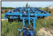
LANDOLL 2210 front & rear disks, 9 shank disk ripper, tandem walking beam axle. S: 25G0900073
