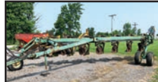
JD 3710 7 BOTTOM ON LAND PLOW , var. width, auto reset, coulters, S: N03710X000382
