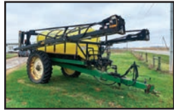
2007 Bestway Field Pro IV pull type sprayer, 90 ft. Boom, hyd pump, 5 section, 3 way nozzle body, 20" spacing, induction cone, rinse tank, Raven 450 w/ Accuboom
