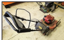
Toro Recycler Push Mower, 22", Briggs & Stratton 7.25 HP Engine
