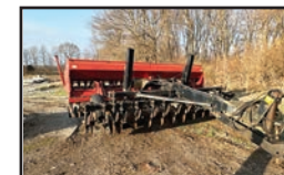
15' Case IH 5400 Drill, no-till cart, 7" spacing
