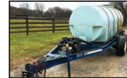
1000 Gallon Duo Lift Nurse Trailer, 8.25 HP Briggs & Stratton engine, 2" plumbing
