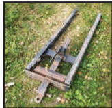
Drawbar hitch assembly , Bolt on/weld on
