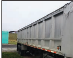
1980 City 30 ft aluminum coal bucket 11R24.5 tires, 5 ft deep dump bed 8 ft wide, 9.5 ft height
