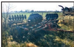
20' Massey Ferguson disc , tandem axle, notched blades on front gang, hyd. fold
