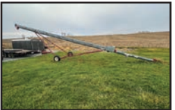
Hutchinson 8"x53' auger, 10 HP elec. motor
