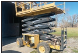
Grove Manlift model SM4688XT, Kubota LP/gas eng., 12-16.5 tires, 927 hrs., excellent cond., lifts over 40 ft.
