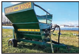
Bale King Vortex Bale Processor 3000, 1000 pto, fine cut option, good hammers
