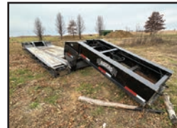
1995 Rogers 35 ton low-boy trailer , wet line detach, 23'6" well, air ride
