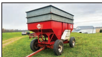
E-Z Flow 400 Bu Gravity Bed, w/ extensions, J&M 12 ton running gear, center divider - each side holds 200 bu clear to the top, 10.00-20 tires. David Stickney, Hillcrest Farms, 937-926-0506, South Vienna, OH
