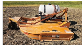
6' woods BB720 rotary mower , 3pt hook up, 540 P.T.O., with hydraulic driven spot sprayer attachment, SN# 10006514426014
