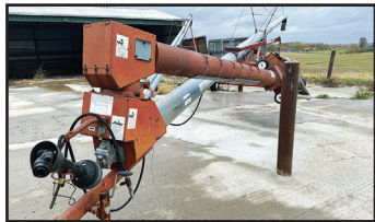
10x62 Mayrath Swing Away Auger, 540 pto, hyd. raise & lower, 235/70R15 tires, SN: 422719. Edward Beeler, 513-616-5613, Hamilton, OH
