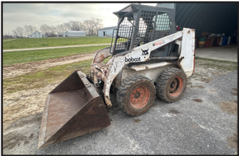
753 Bobcat Skid Steer, 10-16.5 tires, diesel, 66" bucket, auxiliary hydraulics, 3,090 hours, Kurt Hamilton, 937-708-0973, Leesburg, OH
